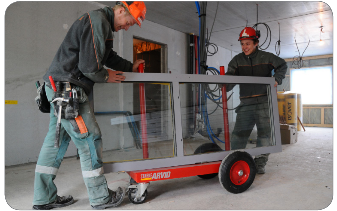
Two swivel castors, one of which is lockable, at the rear
